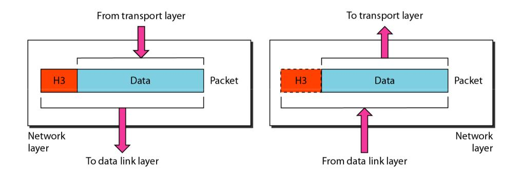
The **network layer** is responsible for the delivery of individual **packets** from the source host to the destination host.
